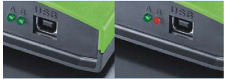
Status indications by means of LEDs on the KTS housing
