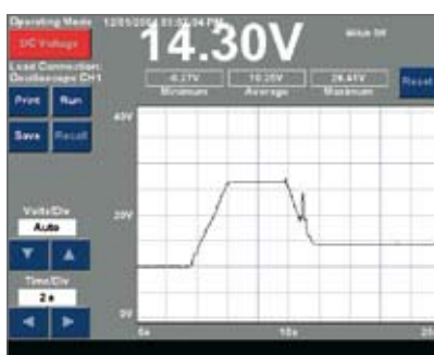
Digital multimeter with graphical and digital display supports rapid evaluation.
